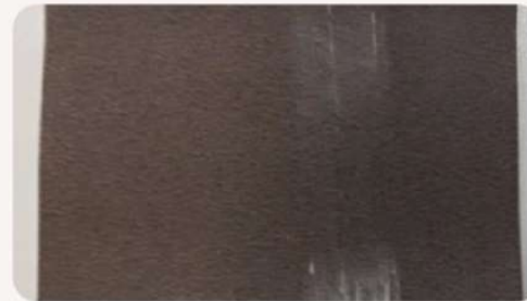
Wallpaper after 500 abrasion cycles - visible scratches
